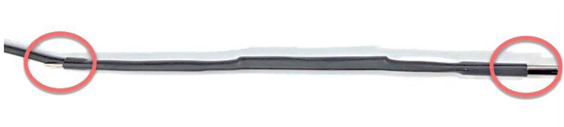
Figure 30. Example of a metal wire protruding from the tube for IP-x7 standard testing.
