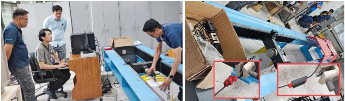
Figure 18. Tensile Test Between Fastening Equipment and Fiber Drop Cable
