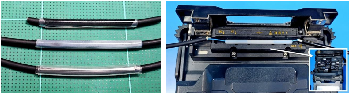
Figure 27. Protection Sleeve quality and heat setting affect the connection point.
