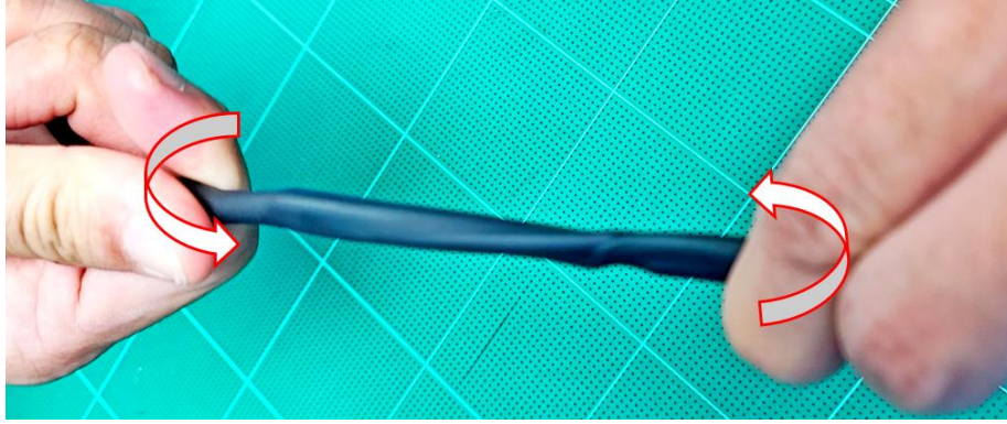
Figure 35. Testing the twisting of the N-MA cable connection point for short-range open FTTx cable.
