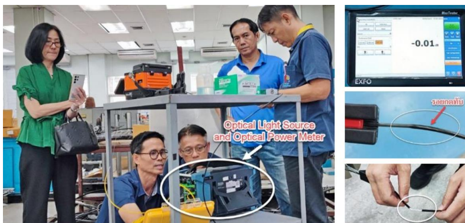
Figure 19. Optical Signal Fed Throughout the Test and Display of Damaged Samples from the Test
